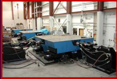
NEES triple biaxial shake tables at University of Nevada, Reno
