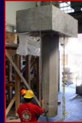
Tests on pile-deck connections at UW
