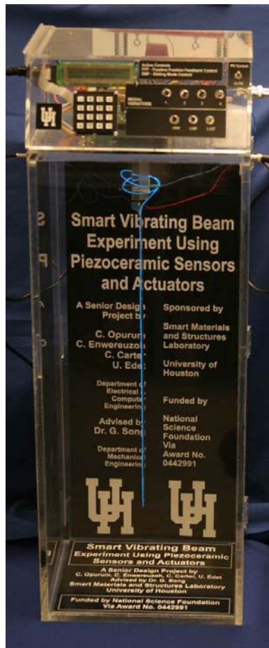
Fig. 1 A portable smart flexible beam with piezoceramic sensor and actuator
